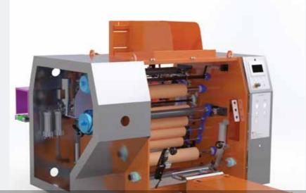
Variant shown: 220 Automatic stretcher with split vari-stretch and return to operator conveyor, built for up to 1000mm wide master roll material
